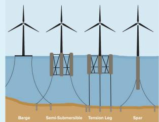
Barge, Semi-Submersible, Tension Leg and Spar. The foundation type will be decided on during the wind farm design phase.
